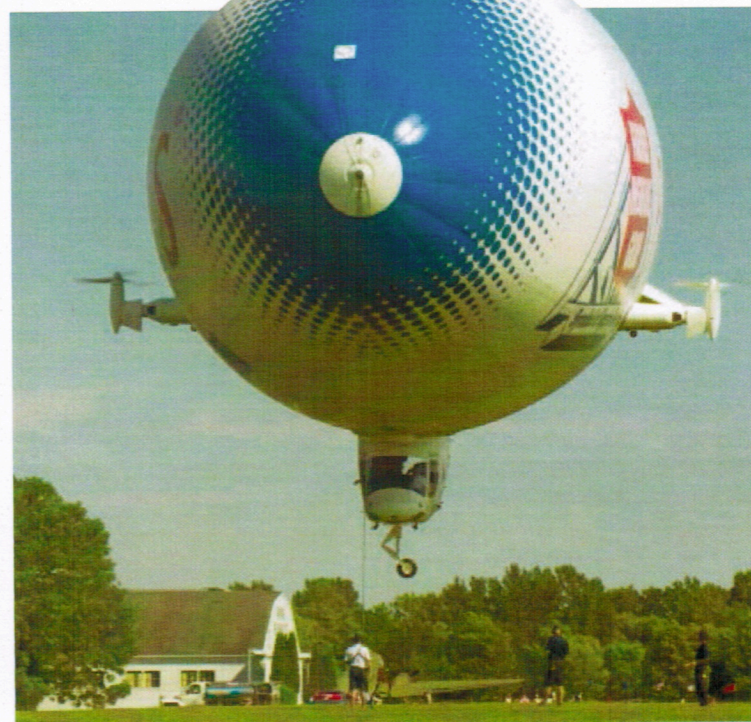
The Farmers Airship comes in for landing like a helicopter, with its side engines vectored 90 degrees up, requiring only three ground crew for assistance.
