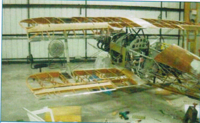
The squared wing tips and larger ailerons provide a faster roll-rate and more stability at slower speeds.
